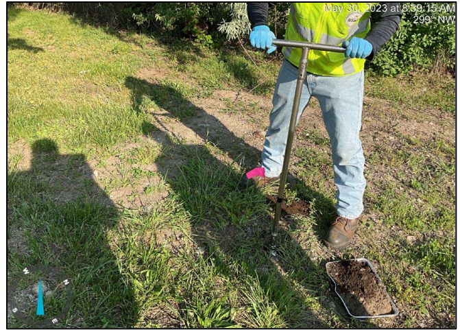
Figure 1 shows an EPA contractor grabbing a soil sample to test it for heavy metals such as lead and cadmium.
